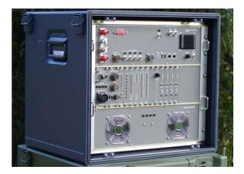
Figure: Customised Digital Broadband-Jammer (Example)
